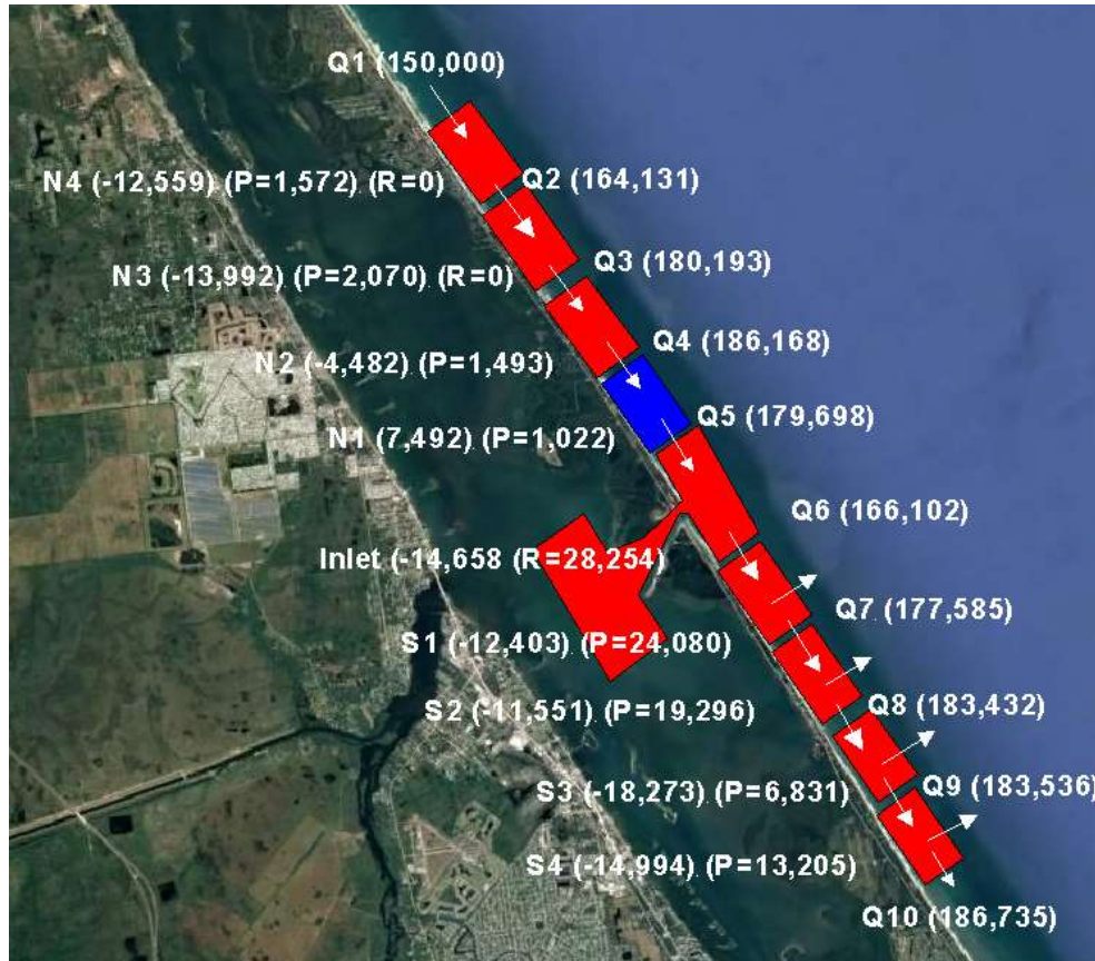
Figure 26. Annualized 10-year sediment budget for the summer 2010 to summer 2020 time period. Values on the west of the barrier island indicate sand volume changes and values on the east indicates calculated sand flux rate in cubic yards per year. P= annualized placement quantities and R = annualized value of sand removed from the sand trap. Blue cells indicate sand volume increase whereas red cells indicate sand volume loss.
