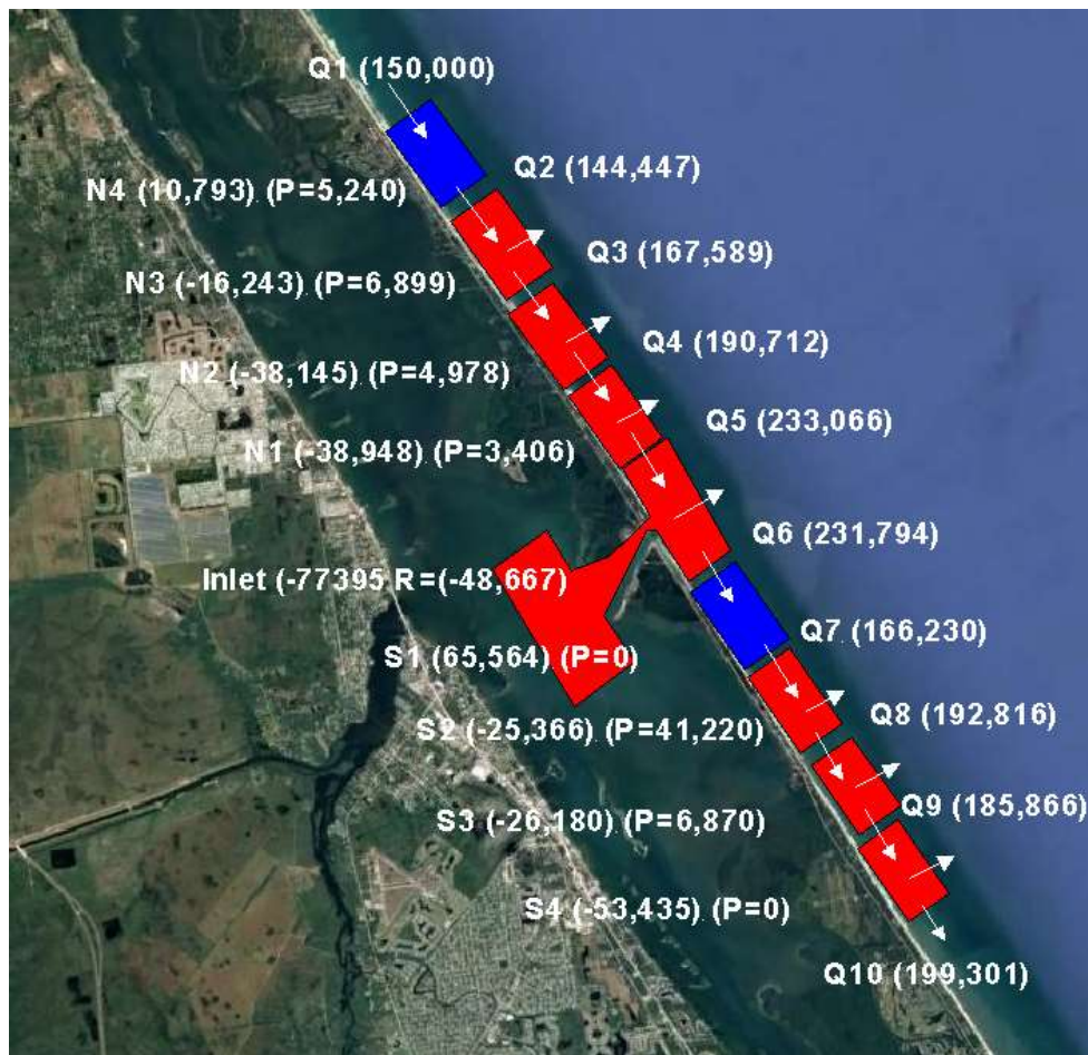
Figure 29. Annualized 3-year sediment budget for the winter 2017 to winter 2020 time period. Values on the west of the barrier island indicate sand volume changes and values on the east indicates calculated sand flux rate in cubic yards per year. P= annualized placement quantities and R = annualized value of sand removed from the sand trap. Blue cells indicate sand volume increase whereas red cells indicate sand volume loss. Offshore transport from each of the cells was required to balance the sand budget.
