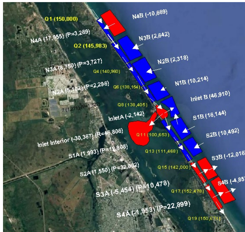
Figure 28. Annualized 10-year sediment budget for the summer 2011 to summer 2021 time period. Values on the west of the barrier island indicate sand volume changes and values on the east indicates calculated sand flux rate in cubic yards per year. P= annualized placement quantities and
